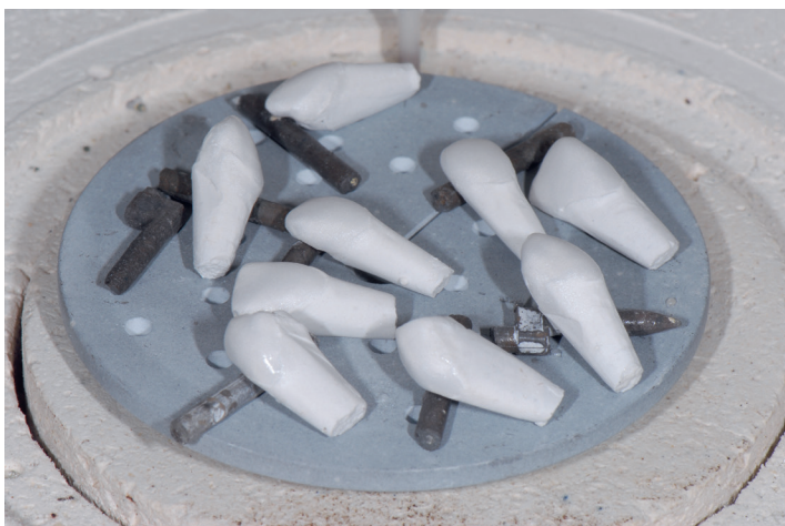
Fig. 11 — It is important that the layered ceramic does not contact the fracture support or adjacent die. The use of absorbent cotton is not recommended as it draws heat away from the dies and leads to too low a firing temperature.
