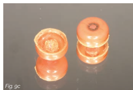
Figs. 9a - c: Titanium nitride coating wear with angled implant in the upper jaw (a). Deformation of nylon Locator matrices with consecutive retention loss (b, c).
